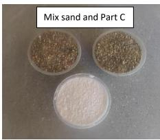
Mix 1 gallon of Part C to 2 gallons torch or oven dried concrete sand.
