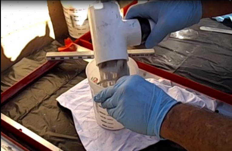
1. Pour 1 measured scoop of part C/sand.
